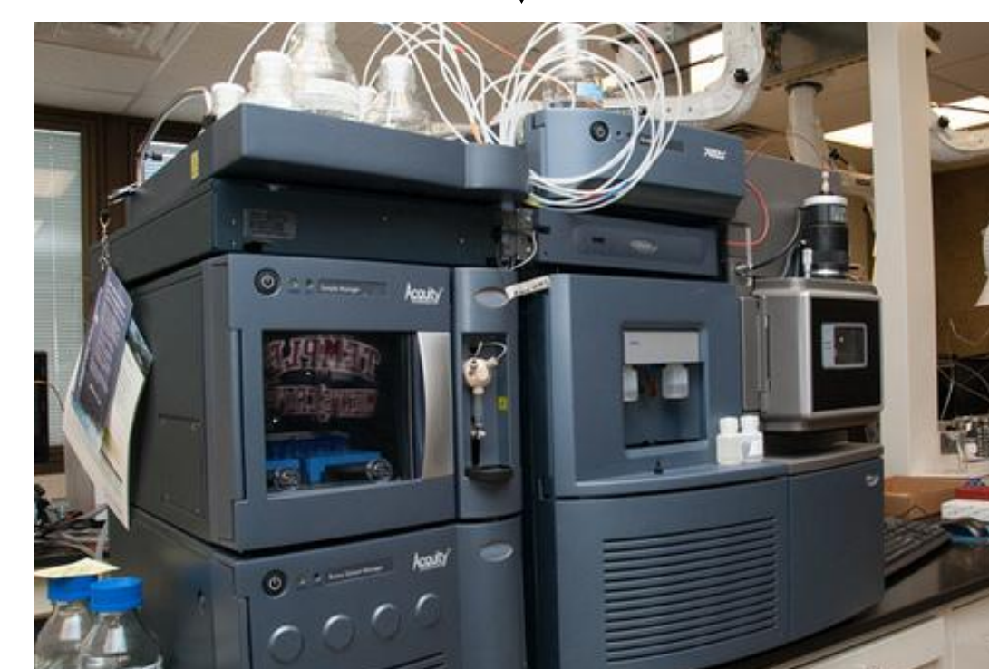
Figure 2. Photo from the WET Center lab showing analytical instrument WATERS XEVO TQMS
