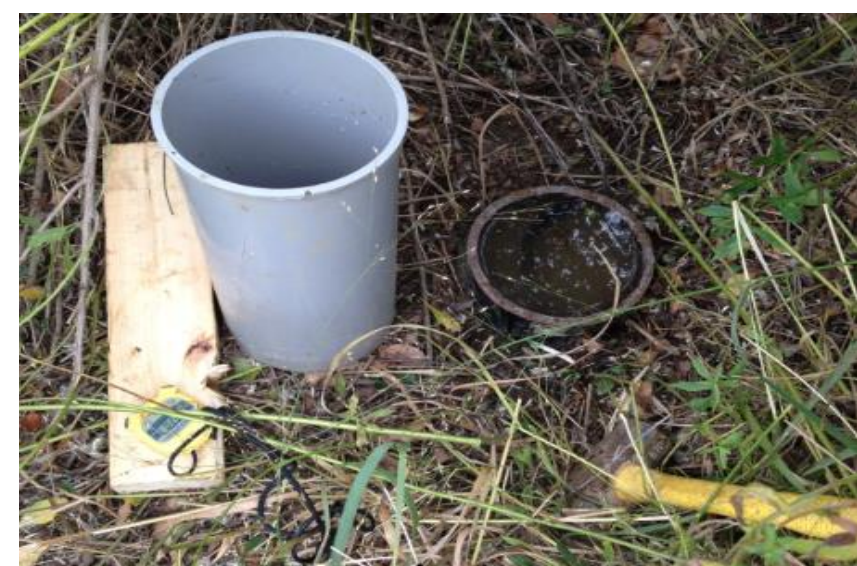
Figure 1: A single-ring infiltrometer test.
