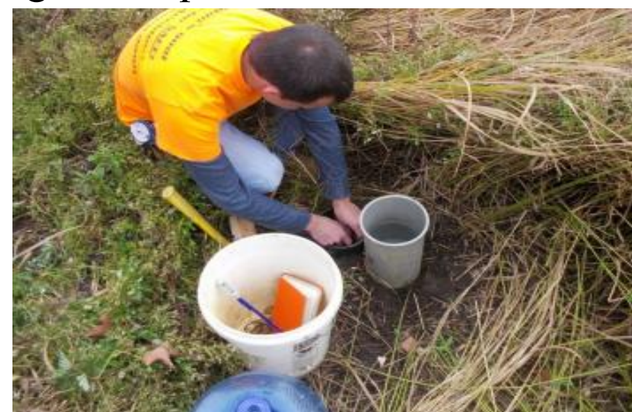
Figure 2: Single-ring infiltration testing.
